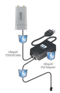
TERMS OF USE: Ubiquiti radio devices must be professionally installed. Shielded Ethernet cable and earth grounding must be used as conditions of product warranty. TOUGHCable is designed for outdoor installations. It is the installer's responsibility to follow local country regulations, including operation within legal frequency channels, output power, indoor cabling requirements, and Dynamic Frequency Selection (DFS) requirements.
